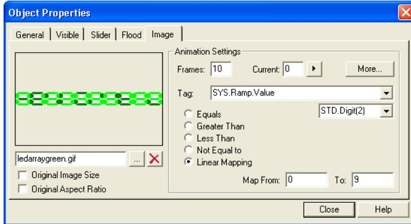
Duplicate the display and position the graphic to the left of the first graphic as shown below. Edit the properties and change the digit number to 2 ie `'STD.Digit (2)'`. Place a dark panel behind the LED's to improve the contrast then preview the screen in the browser.
