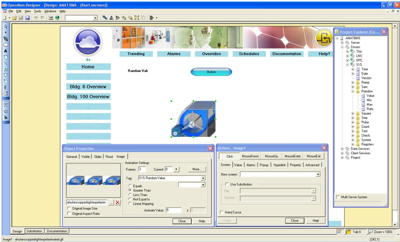
Click on the **Current** button to cycle through the frames and see how the animation will appear. Drag the **Sys.Random.Value** from the Project Explorer onto the Tag and specify the animate value. For this example the fan is required to animate whenever the Sys.Random.Value is greater than 5. Save the screen and validate your results in a Web browser.
