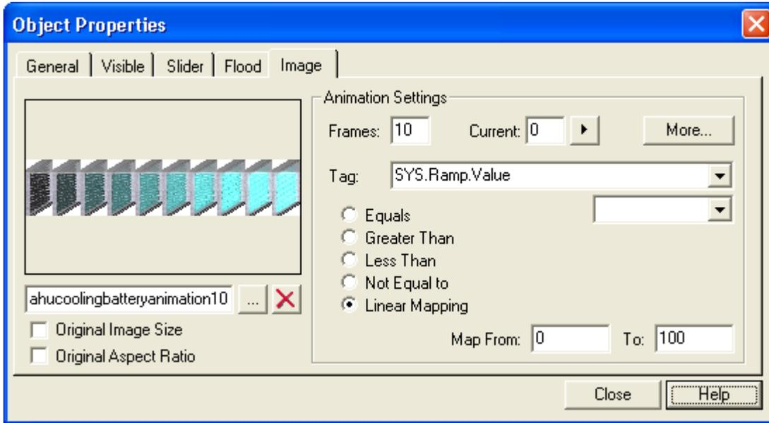
Click on the **Current** button to cycle through the frames and see how the animation will appear. Expand the **Drivers | SYS | Ramp** tree in the Project explorer and drag the **SYS.Ramp.Value** onto the Tag. For the animate value select a **Linear Mapping** from 0 to 100.
