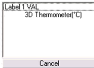
A Temperature Gauge SmartComponent will appear on the screen. Select the Object properties for the SmartComponent and select the **Custom** tab; here you can Change exposed properties of the SmartComponent, in this case the Header Title.
